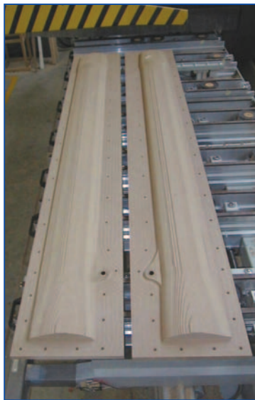
[Fig. 4] - Master in legno del troncone centrale / Wooden master molds for a segment of the mast
